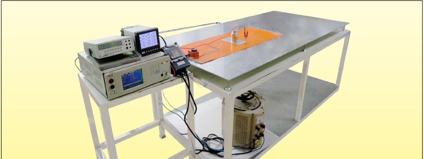
Measuring equipment for total current leakage at hot condition
